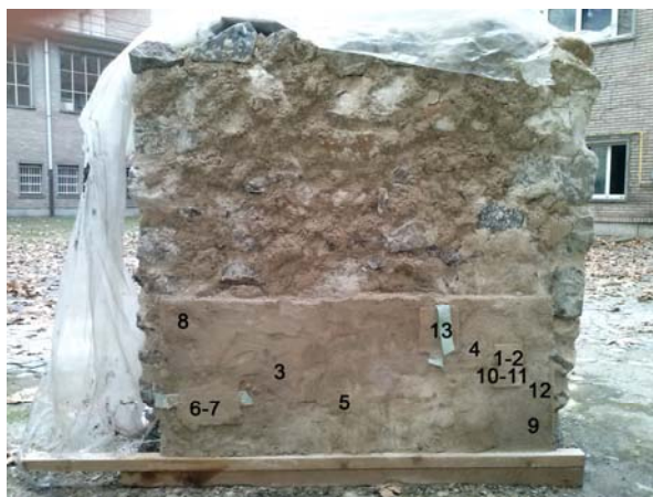
Fig. 3. Position of the measured points on the testing wall.
