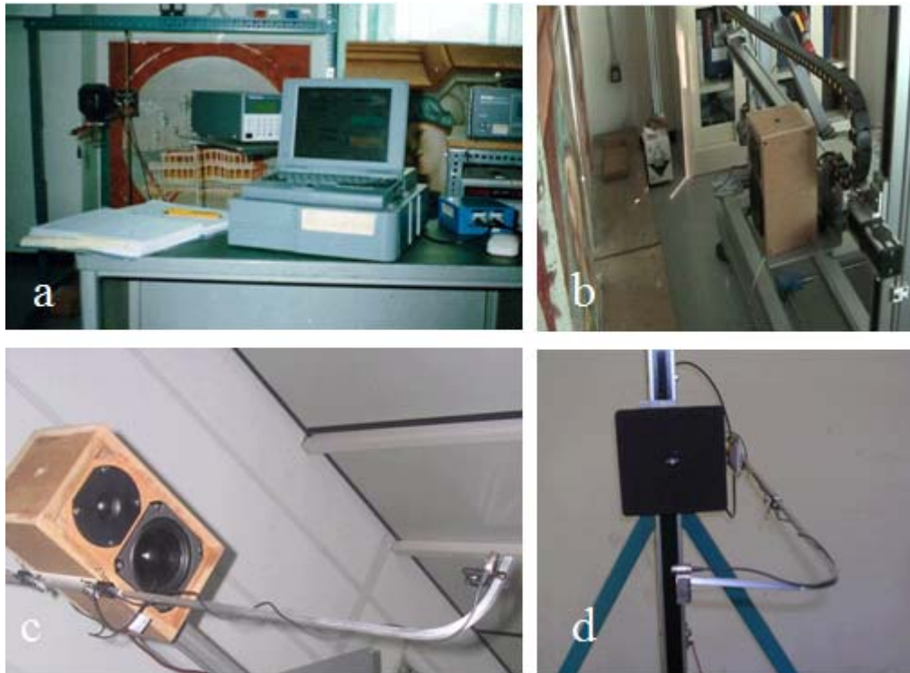
Fig. 2. Advancements in the configuration of the ACEADD system: a – the initial system setup with manual motion of the transceiver unit, during the method laboratory validation (1998-2001); b – part of the 2D automatic system in front of a laboratory model of frescoed surface with detachments; c – transceiver unit with a full range acoustic source and an omnidirectional receiver (2002-2011); d – transceiver unit with a highly directional loudspeaker and an omnidirectional receiver mounted on the linear scan unit (2011-present).
