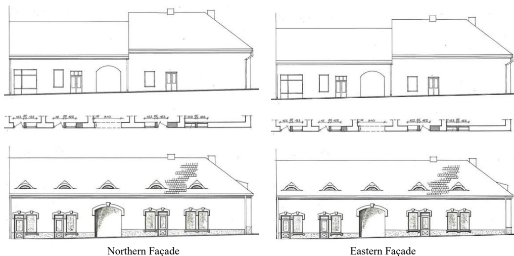
Fig. 12. The condition of the tenement house before the modernization (see above) and the condition of the tenement house after modernization. The visibly designed stairs to the basement have not been implemented.
