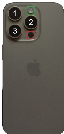
Fig. 3. iPhone 15 Pro with built-in LiDAR scanner (red frame), flash (green frame), and rear cameras (1 – telephoto lens, 2 – ultra-wide-angle lens, 3 – main lens)
