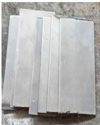
Fig. 1. Lamellae of two types of steel, Laboratory samples, before the hot Forging process
