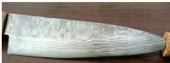
Fig. 4. The "waves" with different color shades as a structural aspect in a sample from the laboratory
