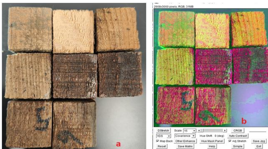
Fig. 12. Wooden samples replica: a) after treatment; b) the effect of the Dstretch YDS filter on the treated wooden samples
