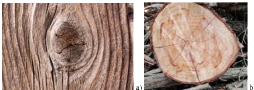
Fig. 5. Example of node (a); shrinkage slot (b)
