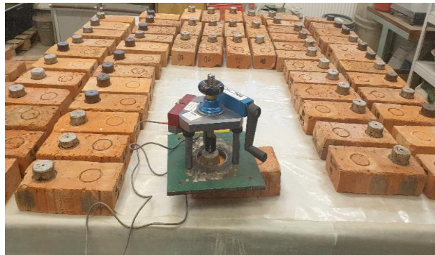
Fig. 4. Conducting a pull-off strength test for bricks
