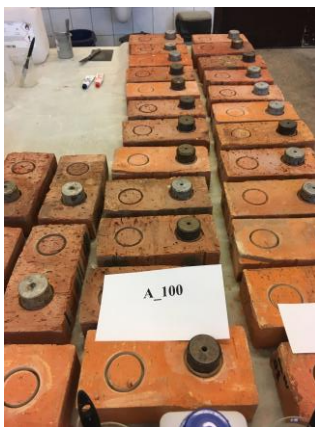
Fig. 3. Inserted pins into the tested bricks
