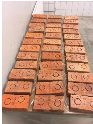
Fig. 2. Cutting the brick and seasoning under laboratory conditions
