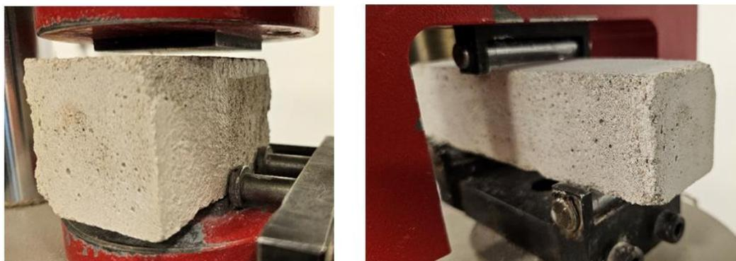
Fig. 1. Mortar specimens: a) compressive test, b) bending test
