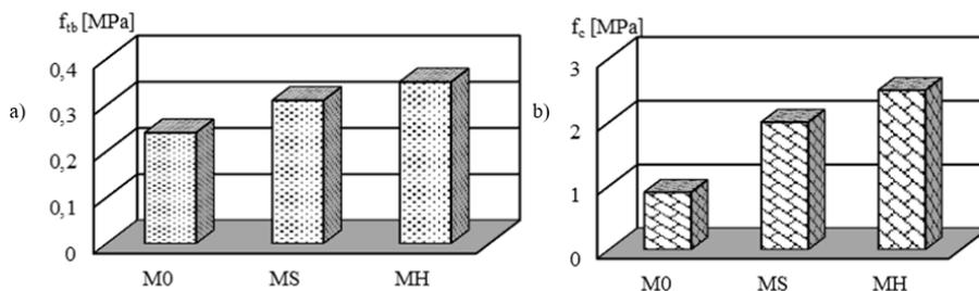
Fig. 3. Strength: a) 3-point bending tensile strength  $f_{t0}$ , b) compressive strength  $f_c$
