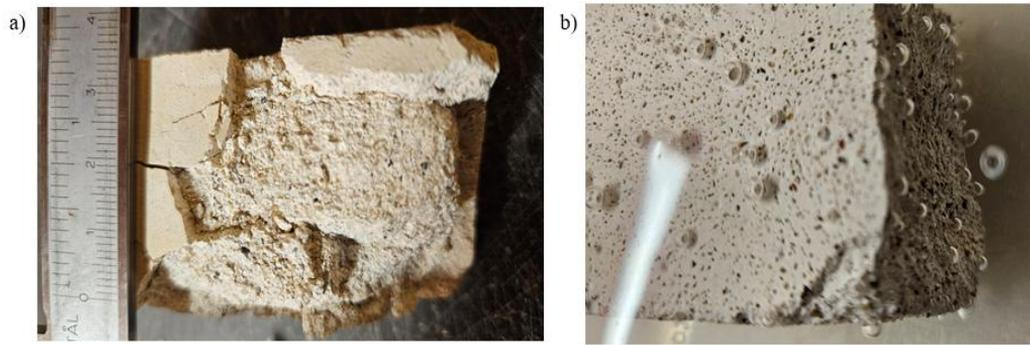
**Fig. 5.** Frost resistance test—general appearance of the lime mortars M0, MS and MH:
