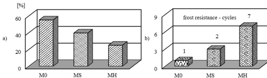
Fig. 2. Tested mortars: a) water absorption, b) frost resistance – number of cycles
