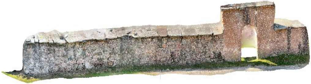
Fig. 2. Example of a visualization of a LiDAR scan of a masonry wall
