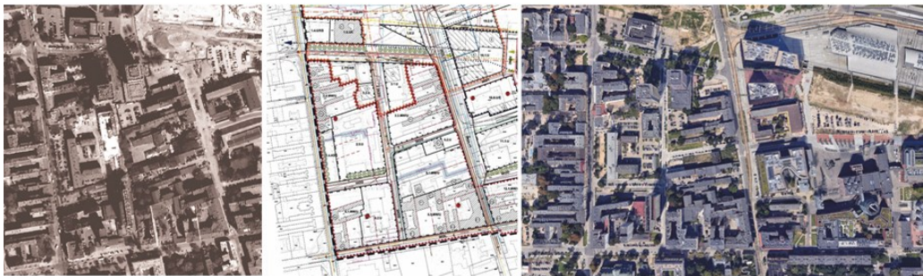
Fig. 3. The Third Revitalization Area (No. 3). An example of a planning document prepared for the needs of the area revitalization process. On the right: orthophotomap, 2016; on the left: local spatial development plan from 2018.
