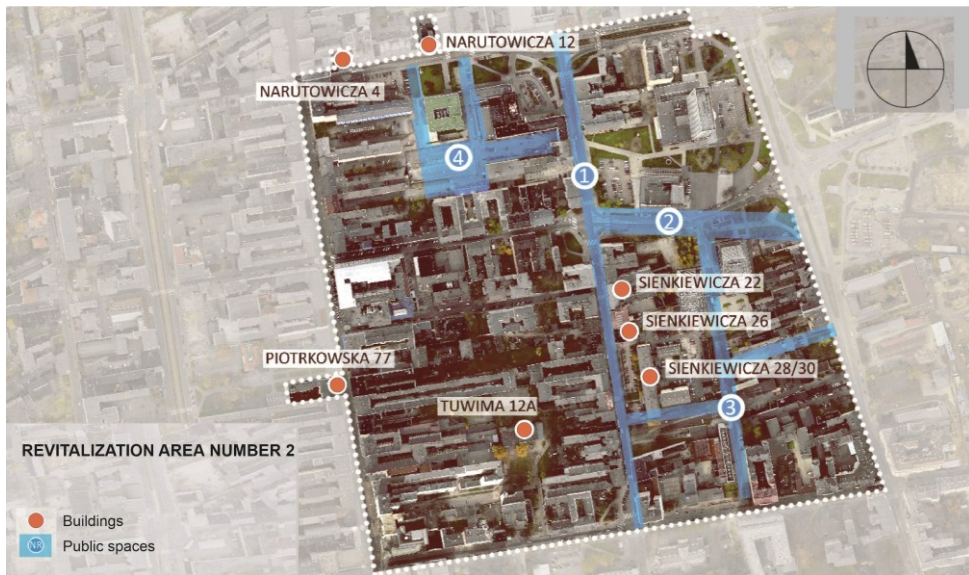
Fig. 11. Scope of investment in Area No. 2 – reconstruction of streets marked in blue and buildings marked with red dots. Construction of a square behind the Polish Television building in the place marked with number 4, the layout of new streets marked with number 3, reconstruction of Traugutta Street marked with number 2, UML graphics, Sources: www.rewitalizacja.uml.lodz.pl [accessed: 03.03.2025]
