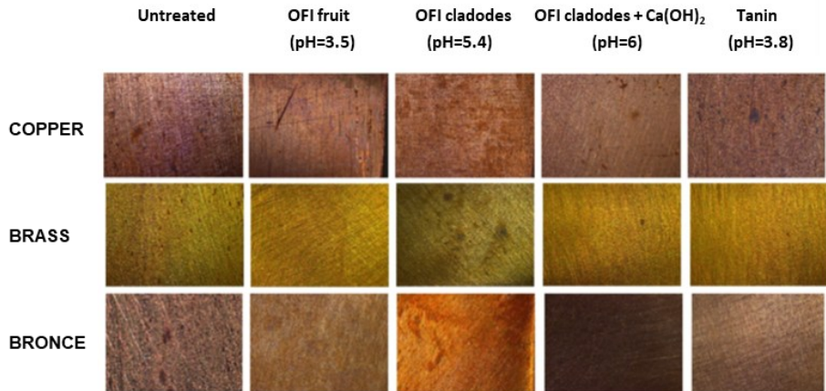
Fig. 4. Microscope images for untreated samples and samples treated for immersion with different extracts
