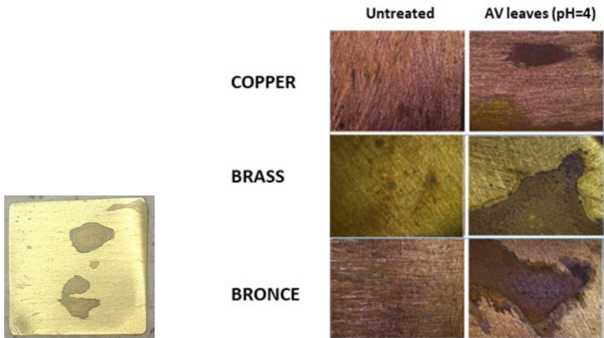
Fig. 2. One example of discoloration on brush-treated sample
