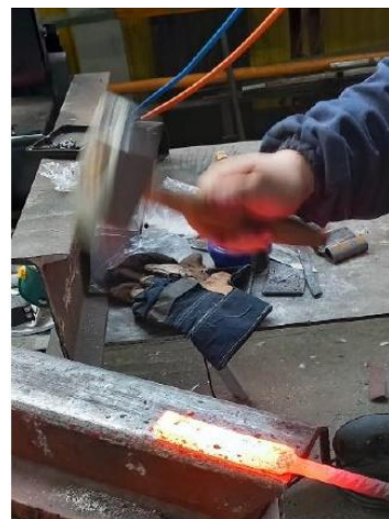
Fig. 5. a). The samples are prepared for forging (Laboratory photo); b). Hot Forging operation
