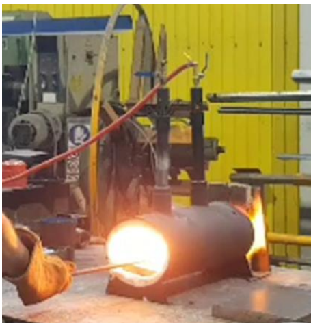
Fig. 5. a). The samples are prepared for forging (Laboratory photo); b). Hot Forging operation
