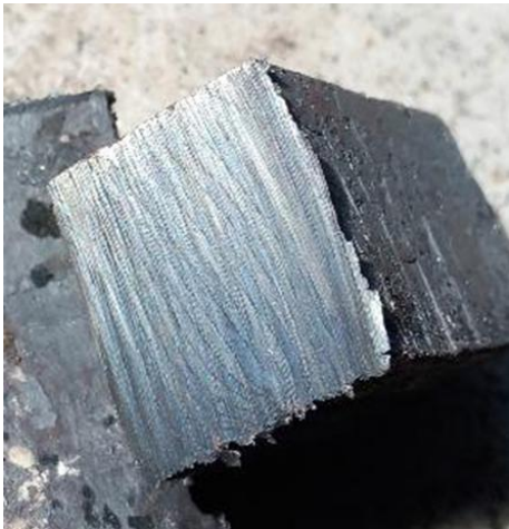
Fig. 6. Damascus steel with 30 layers (laboratory photo), view of the fracture surface, normal size
