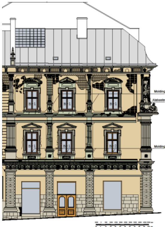
Fig. 6. Cartogram of losses and materials of the Scholtz-Wolfowitz' house at 23 Rynok Square. Facade from the side of Katedralna Square
