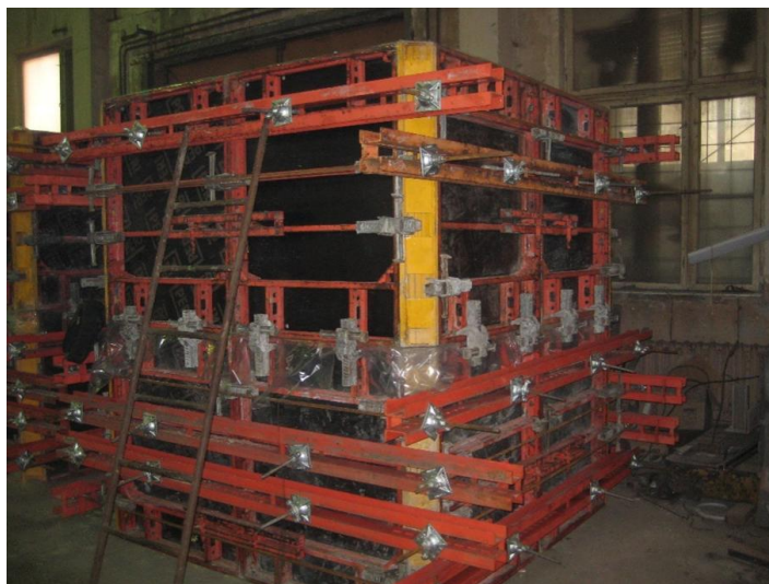
Fig. 10. The limiting structures of the stands are made of formwork.
