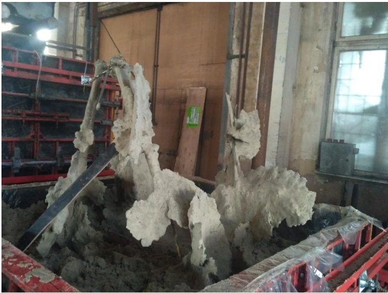
Fig. 13. Stand with removed soil and formed chemical fixation.
