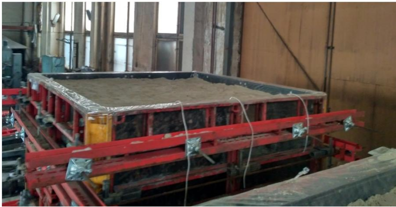
Fig. 11. Sandy soil poured into experimental stands.
