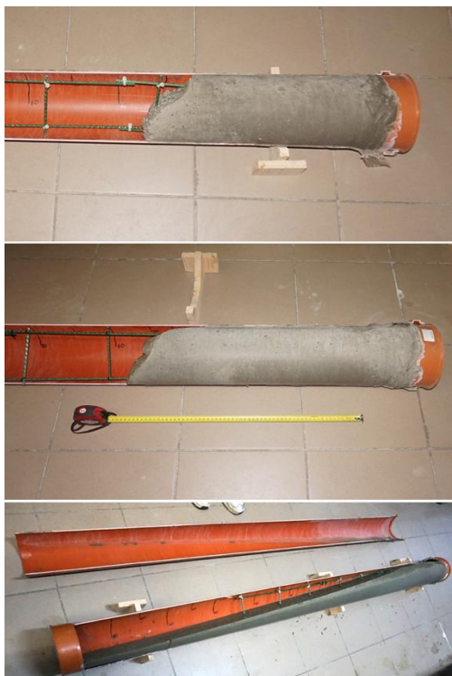
Fig. 8. Results of filling the pipes with concrete mixtures: from top to bottom – mixture No. 1; mixture No. 2, and mixture No. 3
