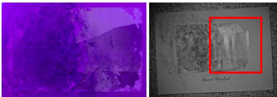
Fig. 19. Examination of the photograph under a UV lamp to investigate the surface (left) and under IR lamp to investigate the surface (right)
