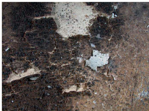
Fig. 12. Stereomicroscopic image showing the paper fibers under the albumen binder at a magnification of 4.7×
