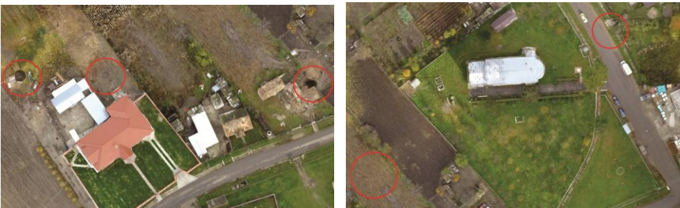
Fig. 8. Identified areas with height differences (image from the drone at a height of 120 m)
