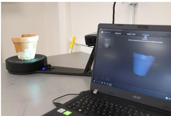
Fig. 8. 3D scanning of a ceramic pot whose pieces are secured with paper tapes
