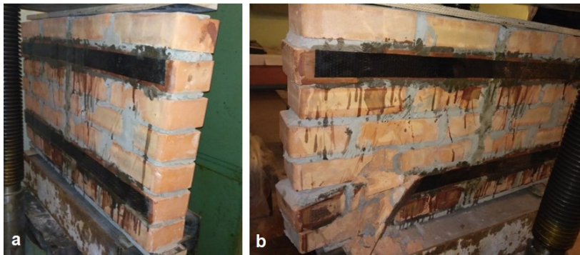
Fig. 9. Experimental studies of brickwork reinforcement with carbon fiber: a – reinforced wall before the start of the experiment; b - the wall after the bending strength test
