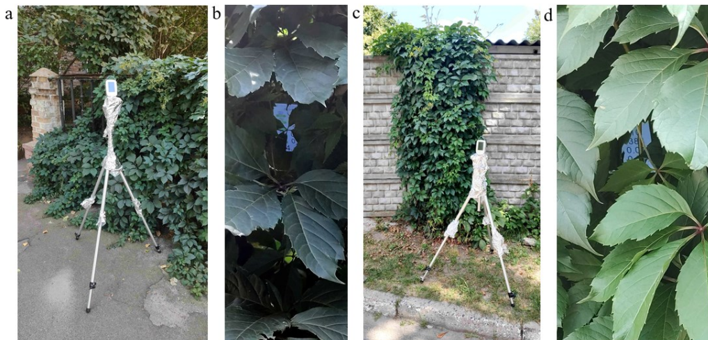
Fig. 8. The field studies of relative humidity around and under the wall greening (authors' picture): a – a blown fence, measuring near to the greening; b – the same, measuring under the greening; c – a solid fence, measuring near to the greening; b – the same, measuring under the greening
