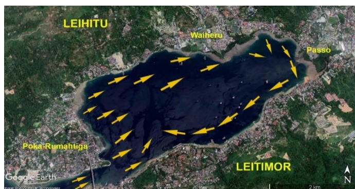
Fig. 8. Tidal current in IAB during tide rises. Drawing based on data from H.G. Saiya et al [15]
