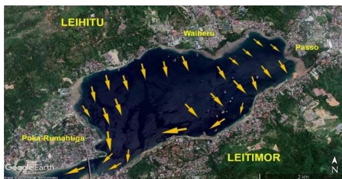
Fig. 9. Tidal current in IAB during tide move down. Drawing based on data from H.G. Saiya et al [15]
