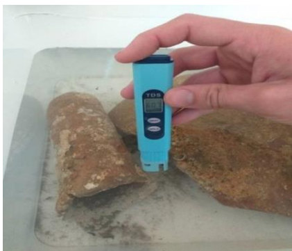
Fig.5. Desalination of two amphora fragments
