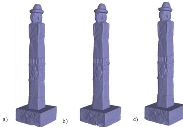
**Fig. 13.** Comparison of solid mesh models created from photogrammetric (a), laser (b) and integrated photogrammetric and laser data (c)
