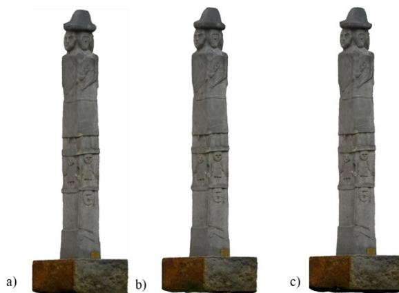
**Fig. 15.** Comparison of final models with textures created from photogrammetric (a), laser (b) and integrated photogrammetric and laser data (c)
