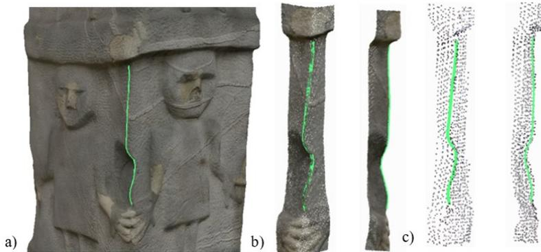
**Fig. 11.** Comparison of the vertical edge vectorised on the mesh model (a) and superimposed on point clouds from photogrammetric (b) and laser measurements (c) shown from two sides
