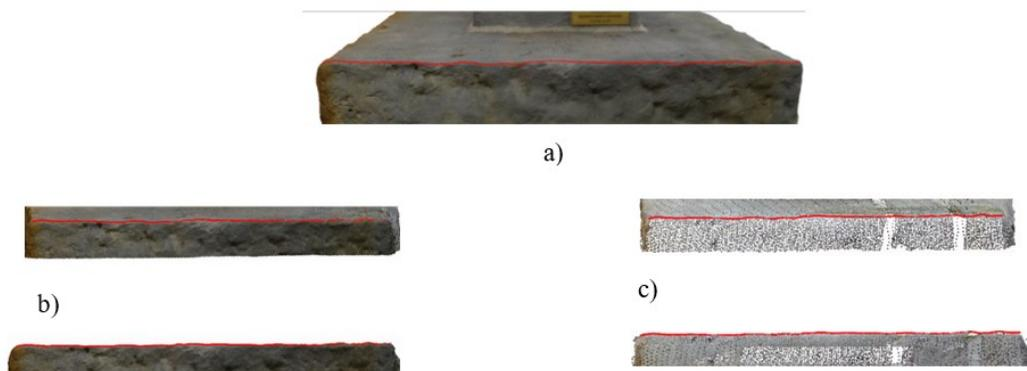
**Fig. 12.** Comparison of the horizontal edge vectorised on the mesh model (a) and superimposed on point clouds from photogrammetric (b) and laser measurements (c) shown from two sides
