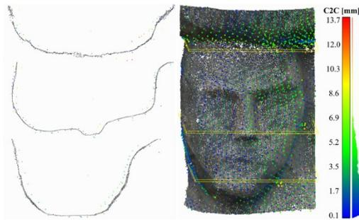
**Fig. 10.** Distances between point clouds determined for surfaces with large depth differences, together with cross sections determined at three locations
