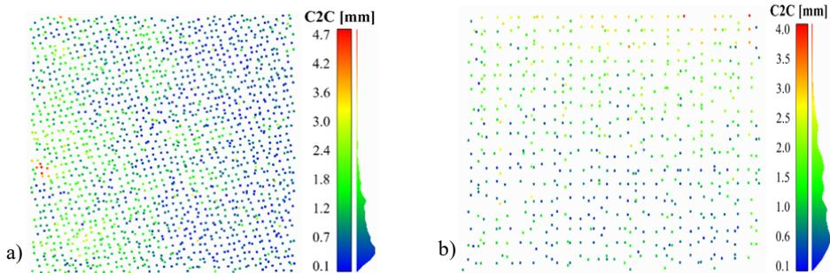
Fig. 7. Distances between point clouds determined for laser data for the study areas before filtering: (a) horizontal surface; (b) vertical surface
