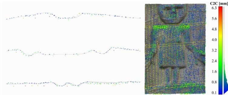
**Fig. 9.** Distances between point clouds determined for surfaces with small depth differences, together with cross sections determined at three locations
