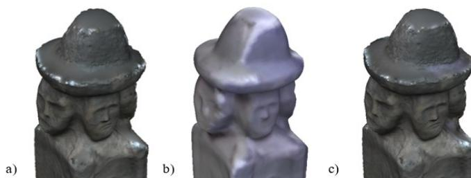
**Fig. 14.** Comparison of the top mesh models created from: photogrammetric (a), laser (b) and integrated photogrammetric and laser data (c)
