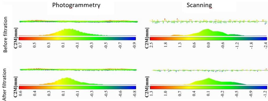
Fig. 6. Comparison of the distance from the fitted plane for a flat vertical surface.
