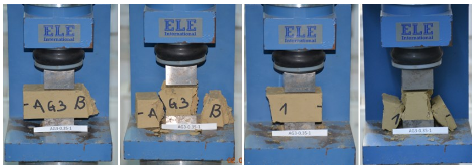
Fig. 4. Compressive strength testing of clay composite (AG3, water/clay ratio 0,4, sample 3 of 6)
