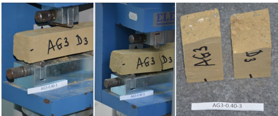
Fig. 3. Flexural strength testing of clay composite (AG3, water/clay ratio 0,4, sample 3 of 6)
