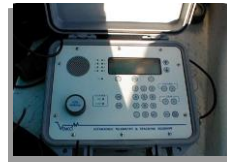
Fig. 7. VR100 equipment for mobile monitoring
