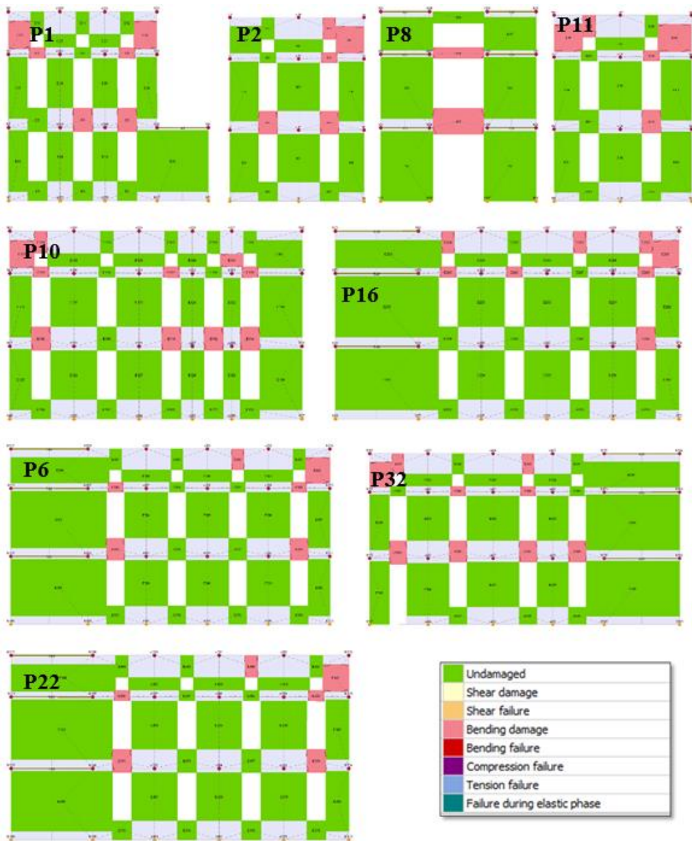
Fig. 22. Damaged walls after pushover analysis in direction +X
