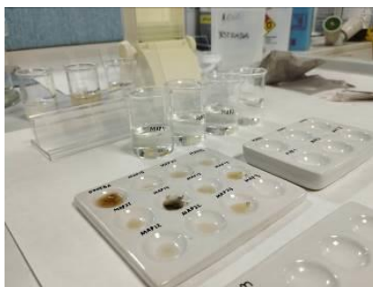
Fig. 2. Fibrous preparations of samples of school maps prior to the microscopic analyses
