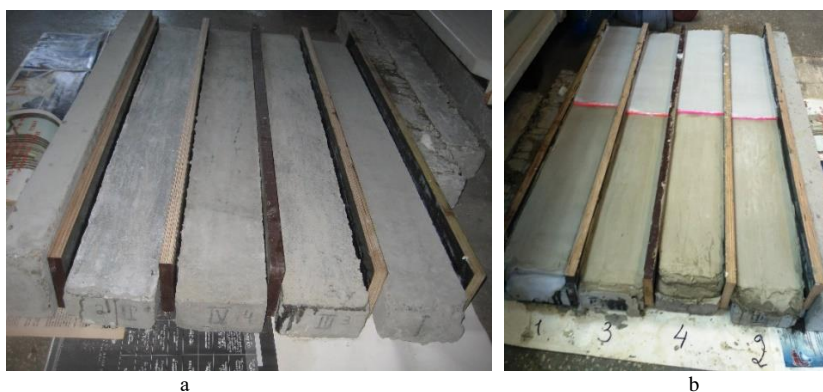
Fig. 9. Lintels for the study of the layers of the structures covering the bicycle track: a – lintels without coating; b – coated lintels
