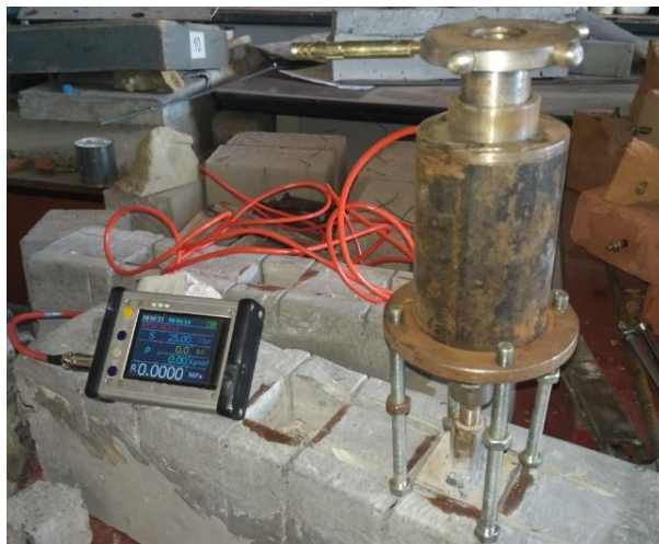
Fig. 11. The process of determining the adhesion strength of structure layers
