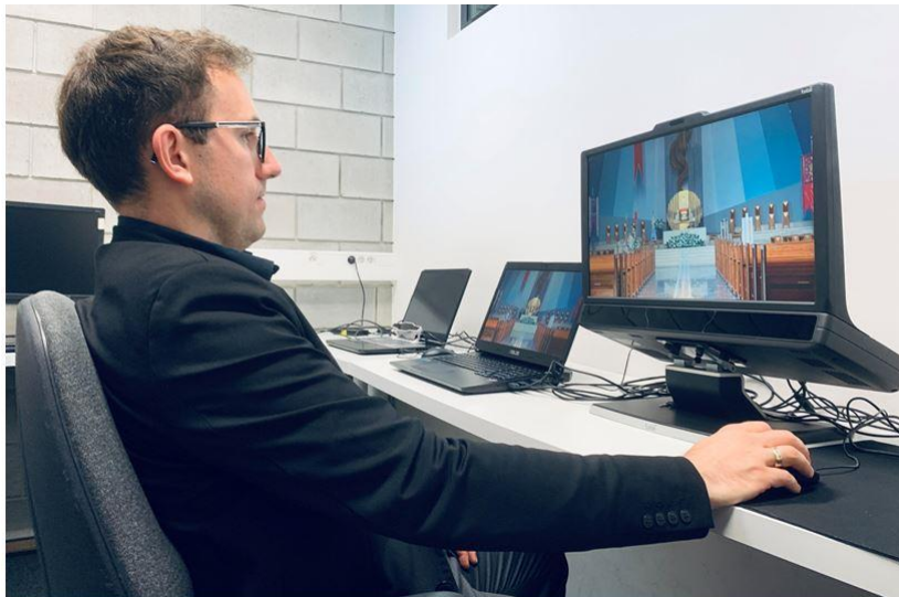
Fig. 5. Photo taken during the experimental study on the remote, binocular video-based eye tracker Tobii TX300
