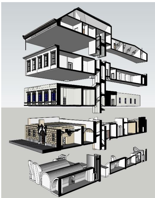
Fig. 4. HBIM model of the building in ul. Kanonicza 1 in Kraków, the seat of the Chair of History of Architecture and Monument Preservation at the Faculty of Architecture of PK (Cracow University of Technology), created on the basis of architectural survey conducted using laser scanning (prepared by Anna Marek, Piotr Pikulski)
