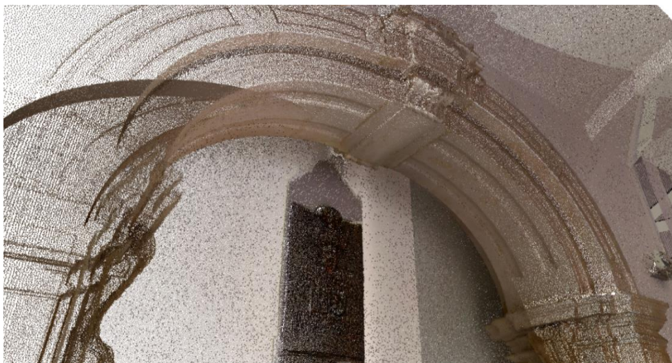
Fig. 3. The laser scan of the historic architectural detail, Łobzowski Palace, Kraków. The point cloud was registered, simplified and imported into the architectural software ArchiCAD
