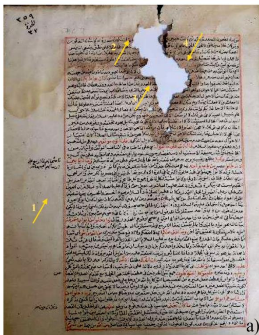
Fig. 4. Measuring spots: a) manuscript M3: 1 - non-degraded paper, 2 - red ink, 3 - black ink, 4 - degraded paper; b) manuscript M4: 5 - non-degraded paper
