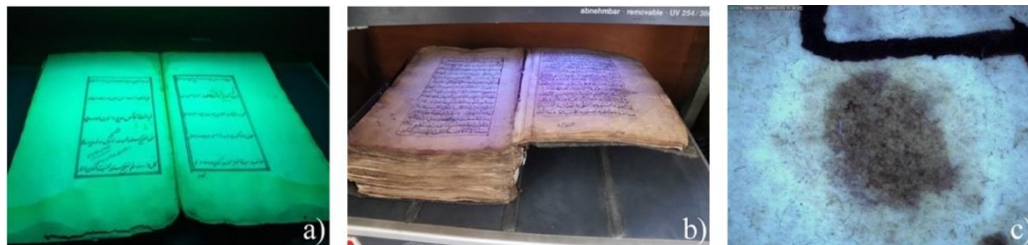
Fig. 1. a) and b) Manuscript pages inspected under UV light, c) 'bull's eye' foxing present in M4 sample
