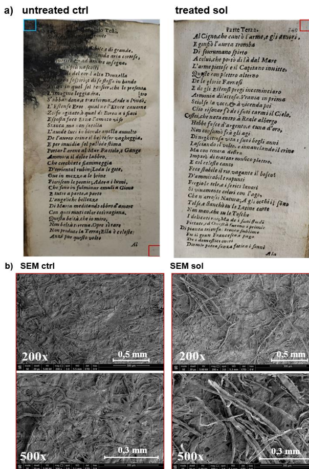
Fig. 2. a) On the left the untreated ink-stained page (untreated ctrl) is shown as reference and represent the extent of the stain on all damaged pages. On the right is shown the ink-stained page treated with commercial products by restorer's direct procedure (yreated sol); b) SEM image of the stained paper with chemical in solution (SEM sol) at 200x (upper image) and 500x (lower image) and relative control (SEM ctrl). A few millimetres have been excised (highlighted in red box in figure a) to perform SEM analysis.
