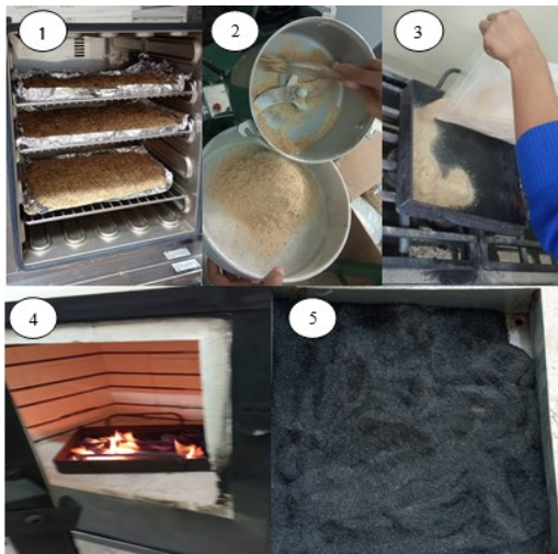
Fig. 2. Rice husk-based biochar production process
