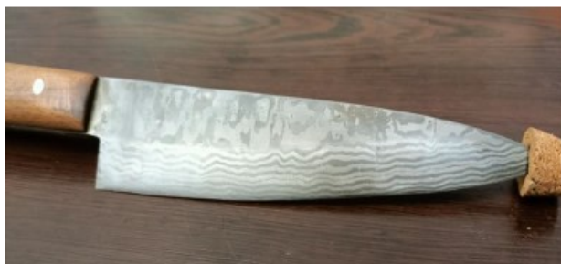
Fig. 7. Damask steel with 30 layers (laboratory photo)
