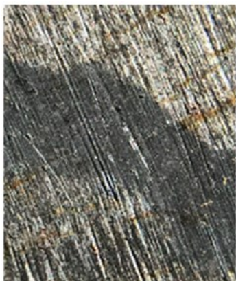
Fig. 10. AISI 1095 steel – the silver area is 15N20 steel
