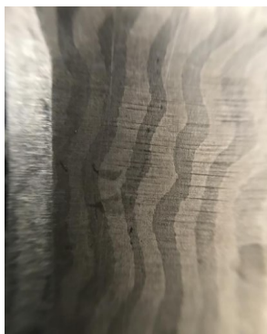
Fig. 6. Special pattern that appears on the blade of the knife
