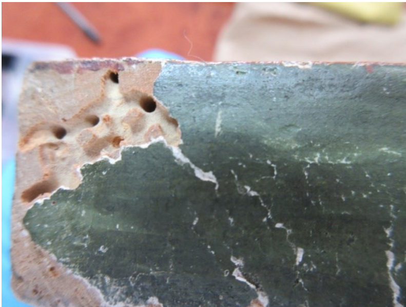
Fig. 10. Simulation of wood-boring damage
