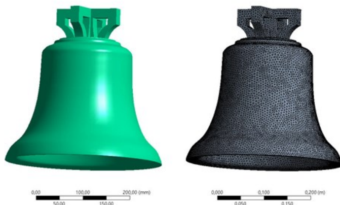
Fig. 2. Geometrical model (on the left) and its mesh (element size: 5mm, nodes: 388078, elements: 203650) (on the right)
