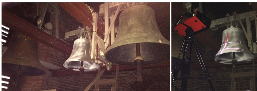
Fig. 1. Bells on the tower in one of the churches in Kudirkos Naumiestis (Lithuania) (on the left) and the process of scanning one of them (on the right)
