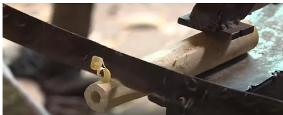
Fig. 8. Construction of the alphorn's mouthpiece
