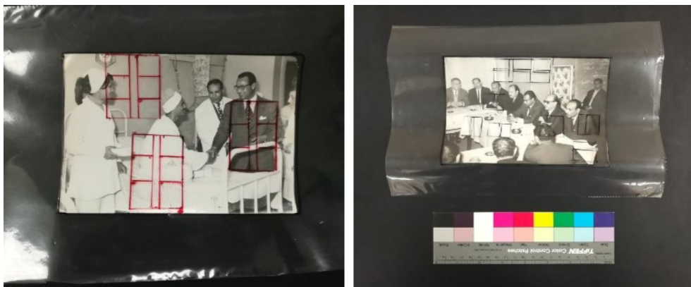
Fig. 2. Shows the selected silver gelatin prints and gel application areas and the selected areas for measuring the optical and chemical properties before treatment, after treatment, and artificial ageing
