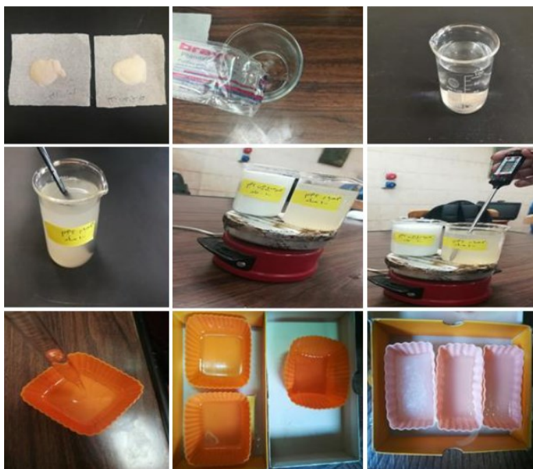
Fig. 3. Gel-based systems preparation steps
