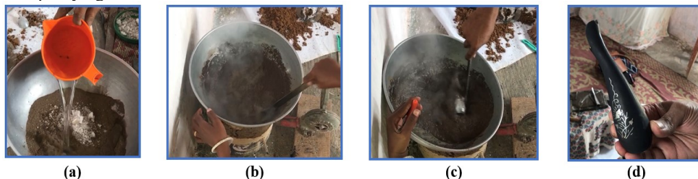
Fig. 3. Oxidation Process of Bidri Handicraft Process: a) Addition of water for clay poultice; b) Boiling slurry on furnace; c) Rolling of artefact in boiling solution (partial patination formed); d) Finished Bidri product
