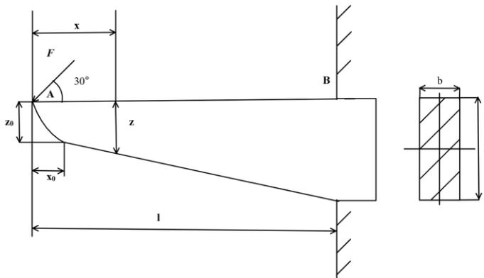
Fig. 7. Beam with variable section of equal strength
