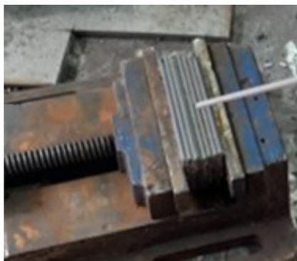
Fig. 1. Alternating the two layers of steels
