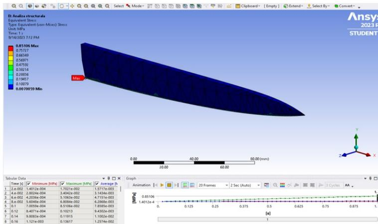
Fig. 15. Equivalent stress, in the case of  $F = 15N$
