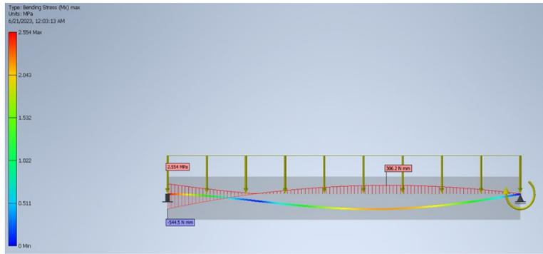
Fig. 8. Indeterminate static analysis [8], for  $F = 20\text{N}$ , Bending Stress in material [MPa]
