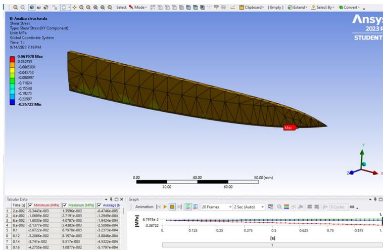
Fig. 14. Shear stress, in the case of  $F = 25N$ : Maximum value is 0.067978MPa
