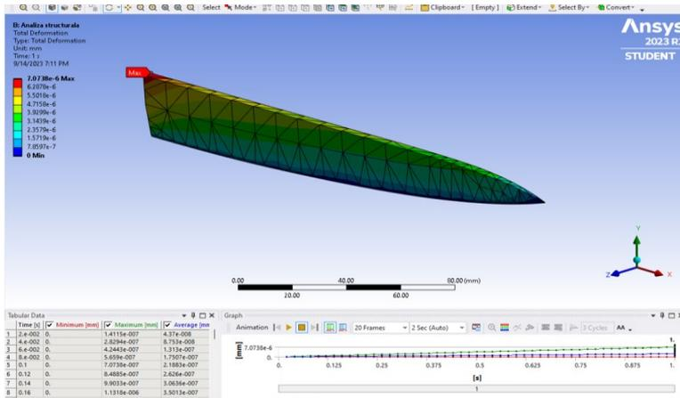
Fig. 17. Total deformation of the knife (0.0000070738mm), for F=15N
