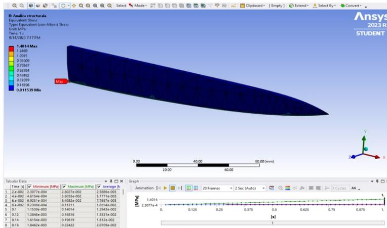
Fig. 16. Equivalent stress, in the case of F=25N
