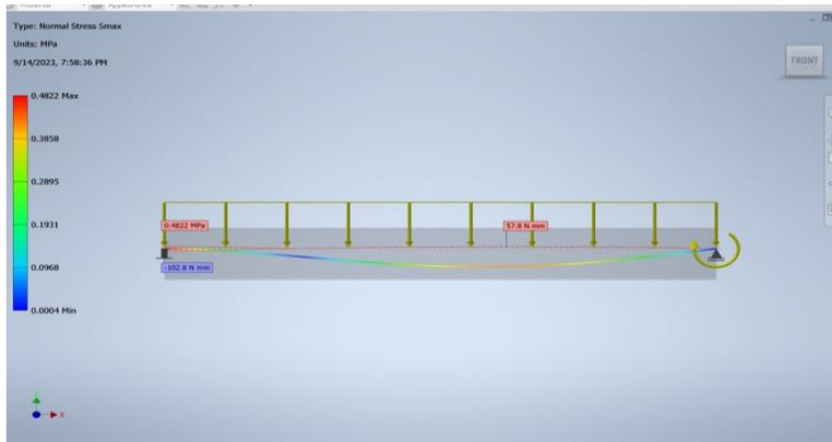
Fig. 9. Indeterminate static analysis, for  $F = 15\text{N}$ , Normal Stress/Tensions in material
