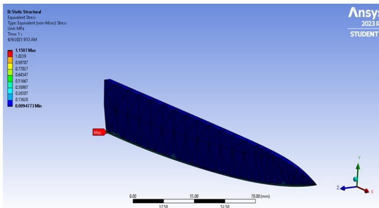
**Fig. 12.** Equivalent stress (von Mises), in the case of  $F = 20N$
