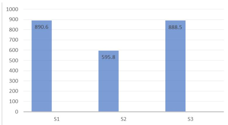
Fig. 5. Evolution of the Vickers microhardness of the Damask steel depending on the treatments S1, S2 and S3
