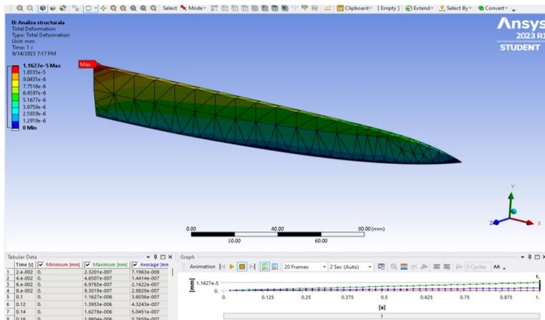
Fig. 18. Total deformation of the knife (0.000011627mm), for F=25N
