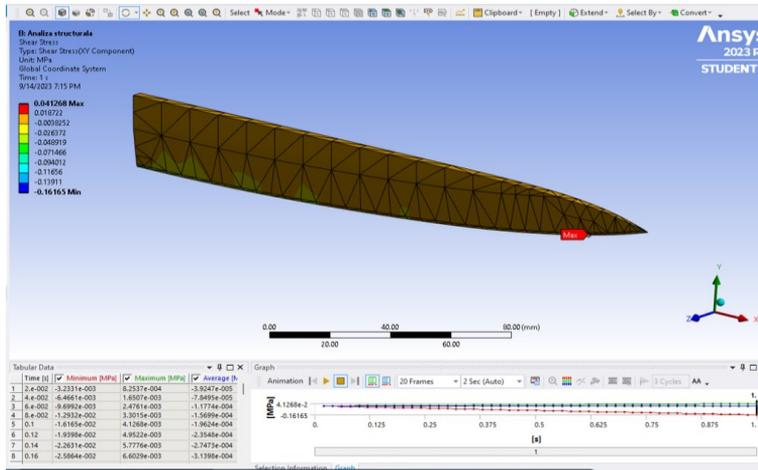
Fig. 13. Shear stress, in the case of  $F = 15N$ : Maximum value is 0.041268MPa
