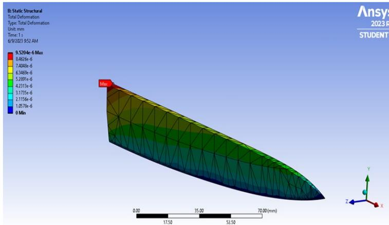
**Fig. 11.** Total deformation (0.0000095204 mm), in the case of  $F = 20N$
