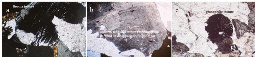
Fig. 6. Petrographic view of the texture of granite in the tombs of Sun El-Hagar: a - Brucite texture; b - ordinary rang texture; c-gianophilic textyre
