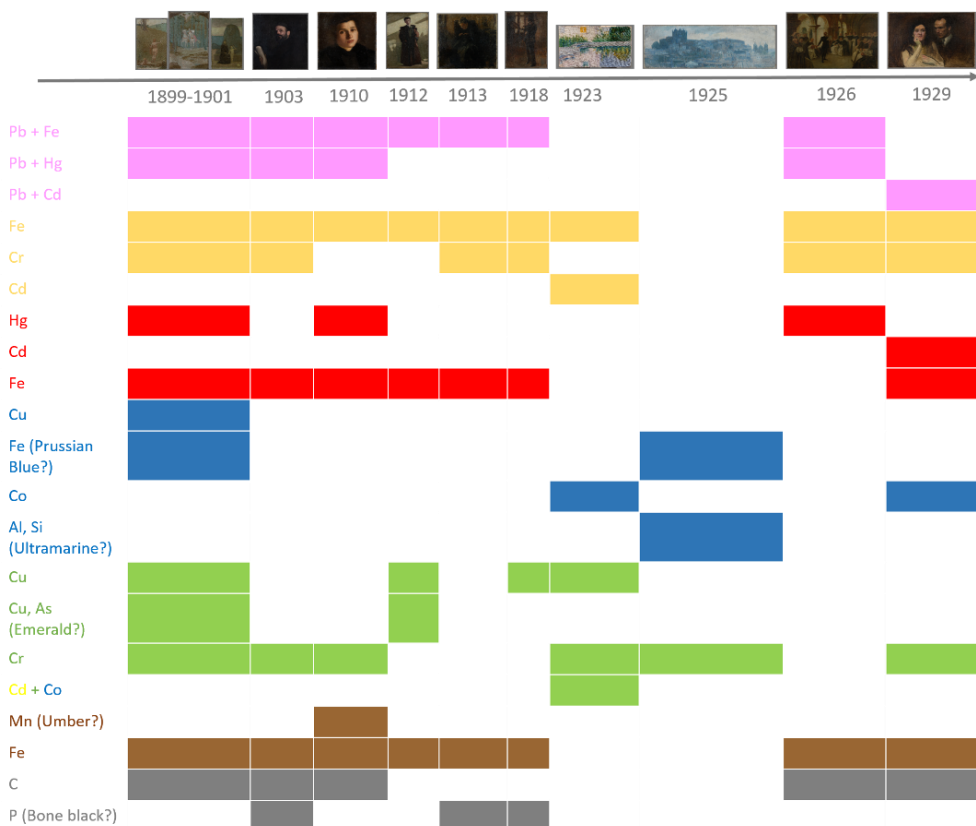
Fig. 15. Summary table of the interpretation of the XRF spectra collected from the chromatic layers
