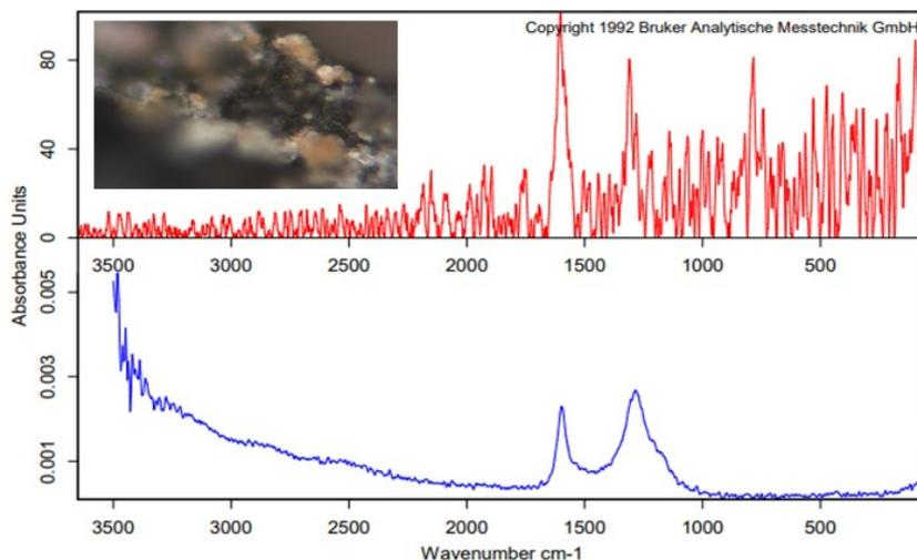
Fig. 7. Raman spectra detected from black pigment
