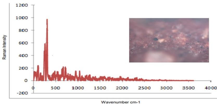
Fig. 9. Raman spectra detected from the red pigment
