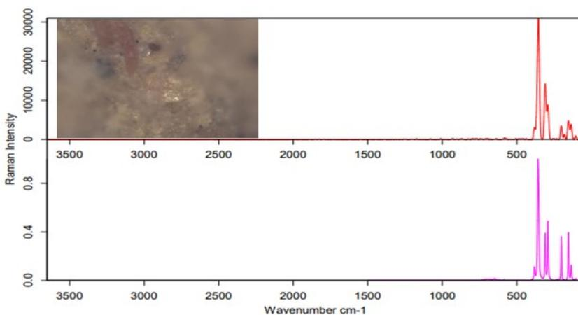
Fig. 8. Raman spectra detected from yellow pigment
