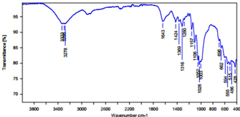
Fig . 11. Transmission FTIR spectra of fabric layer
