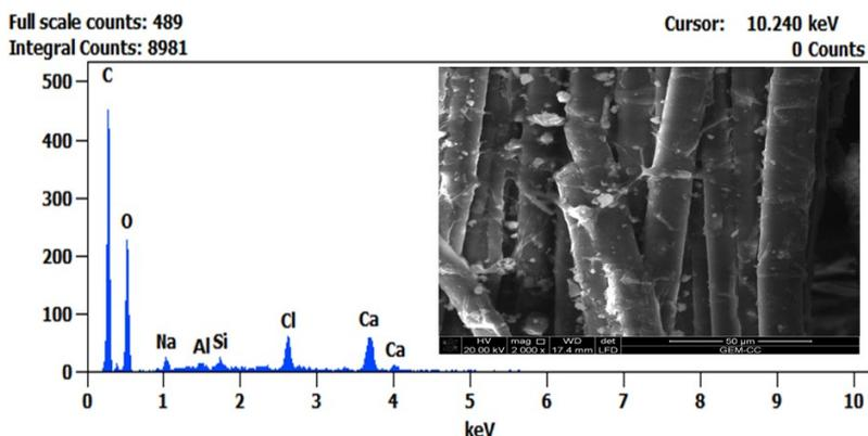
**Fig. 5.** EDS spectrum of linen weave used in the layered structure of cartonnage
