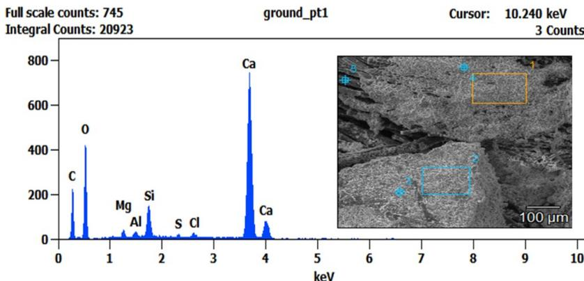
Fig. 6. EDS spectrum of the ground layer
