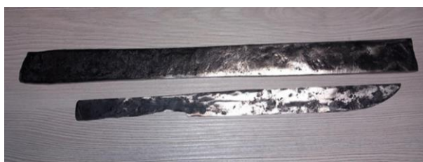
Fig. 8. Damascus steel with 30 layers (laboratory)
