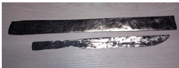
Fig. 8. Damascus steel with 30 layers (laboratory)
