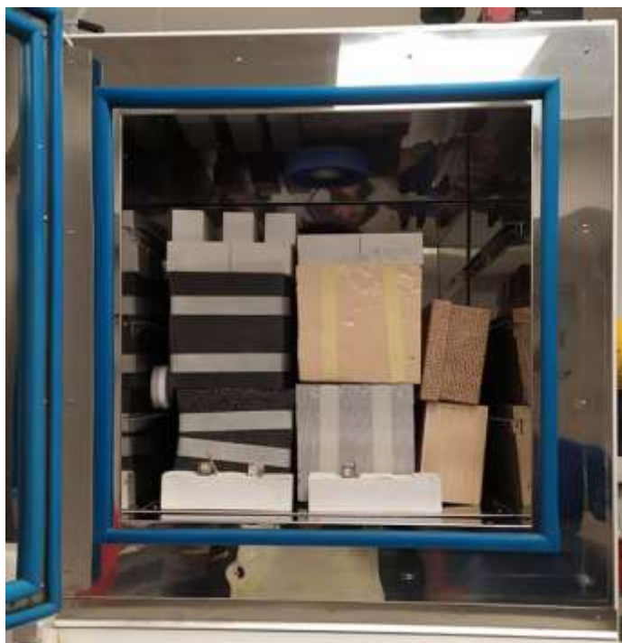
Fig. 2. Climatic chamber uses in the analysis of the prototypes.
