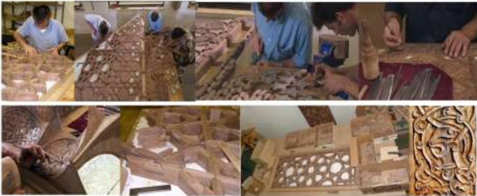
Fig. 16. Pictures showing the reconstruction phases of geometric shapes, muqarnas and biomorphic and inlay designs, (Faculty of Islamic Arts and Architecture at WISE visual library)
