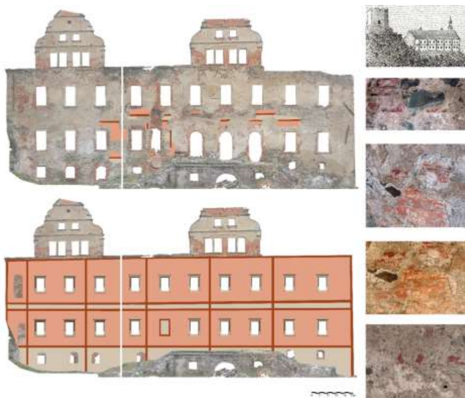
Fig. 5. Niesyto Castle in Płonin. Photo-scan of the southern facade with the remnants of architectural polychromes, and also a reconstruction of the 17th-century color scheme (drawing by M. Chorowska and P. Błonieński)
