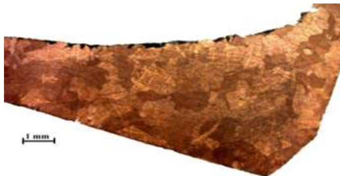
Fig. 3. Photomicrograph Showing Deformed Dendrites, Twins and Strain Lines
