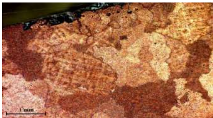
Fig. 4. Photomicrograph Showing Black Globules of Lead
