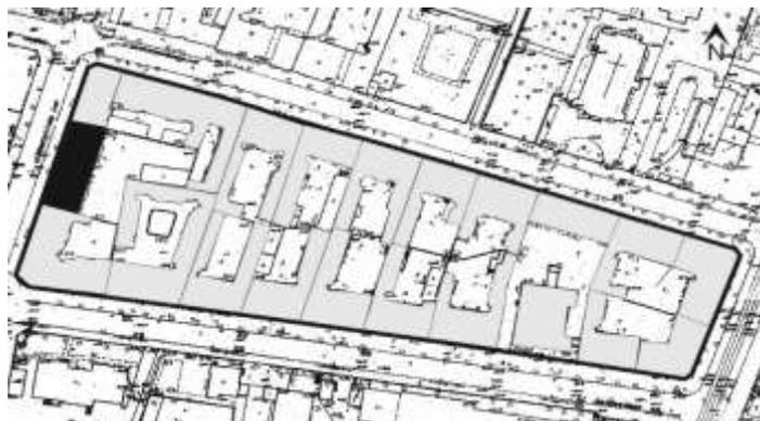
**Fig. 12.** A multi-family residential building from 1960-1964, complementary, at Wawrzyniaka 28/30 street in Poznań. Location in a city block resulting from the implementation of J. Stubben's plan. The existing investment is marked in grey and the complement is marked in black.
